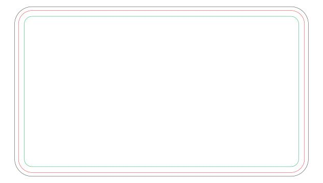
Red line is the die cut Green line is the 3mm safety net Black line is 2mm bleed
